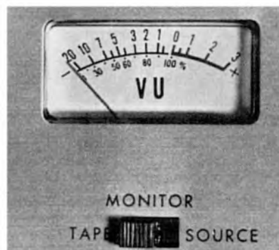
Fig. 3. VU meter and monitor switch on the Truvox recorder
